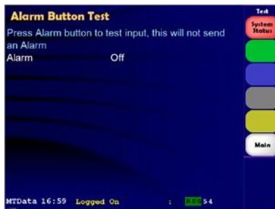
Figure 67: Alarm button test display
